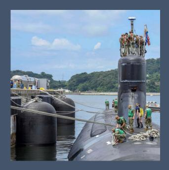
Ocean Guard™ Hydropneumatic Fenders are for vessels requiring subsurface fender contact such as submarines. For the fender to stand vertically, it is partially filled with water, pressurized with air, and finally a counterweight of concrete or steel is added.
